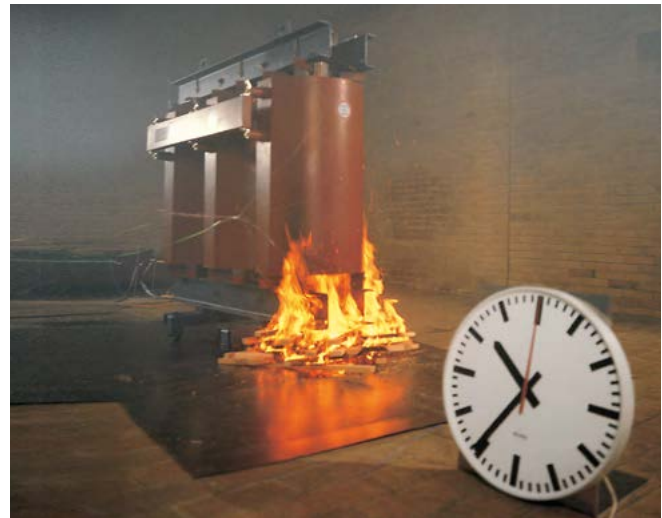
Fig. 5.11-7: Flammability test of cast-resin transformer
