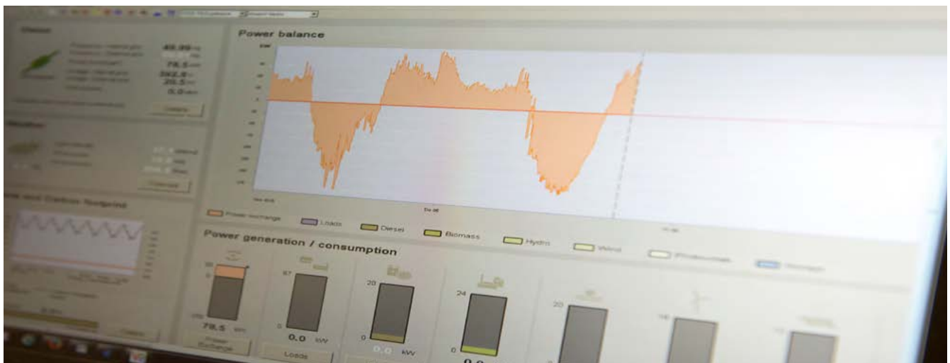
Fig. 2.5-1: Microgrid manager balancing load, generation and storage
