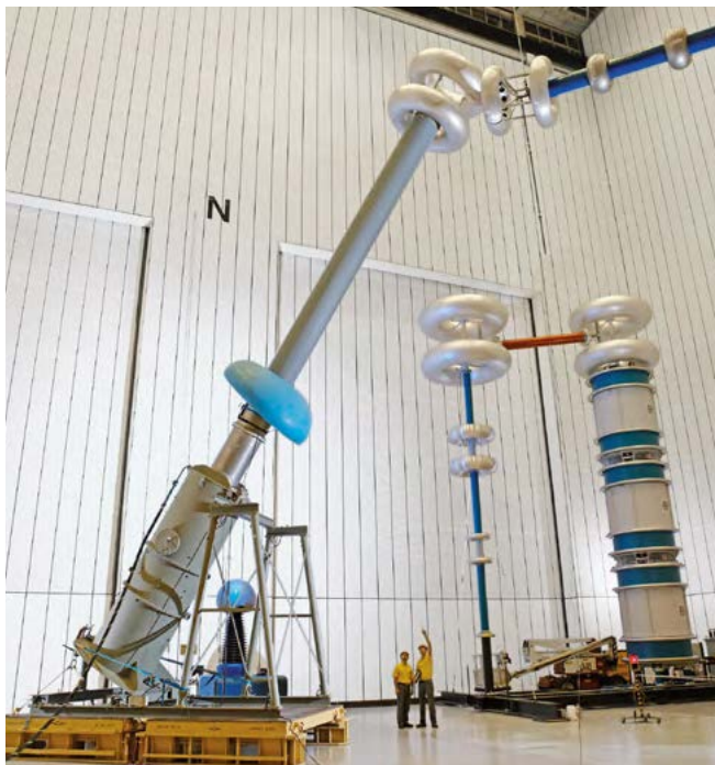
Fig. 4.2-46: Transformer bushing – 800 kV UHVDC – project Yunnan-Guangdong, China
