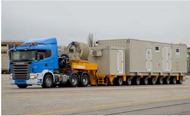
Fig. 2.4-12: 36kV/12kV 16 MVA mobile substation
