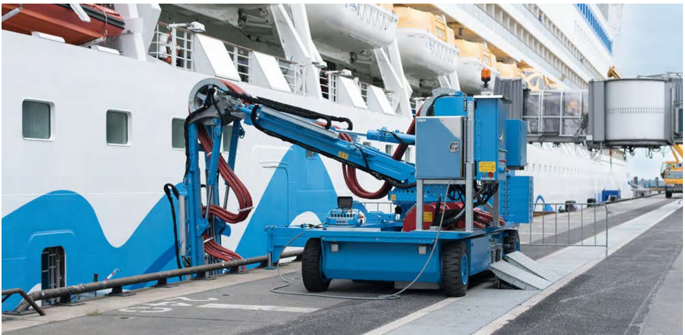
Fig. 2.3-17: Quick and easy connection to the ship via the cable management system
