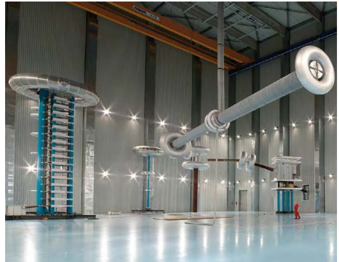
Fig. 4.2-47: Wall bushing – 800 kV HVDC – project Yunnan-Guangdong, China
