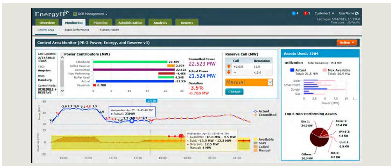
Fig. 7.2-16: DEMS Control Area Monitor
