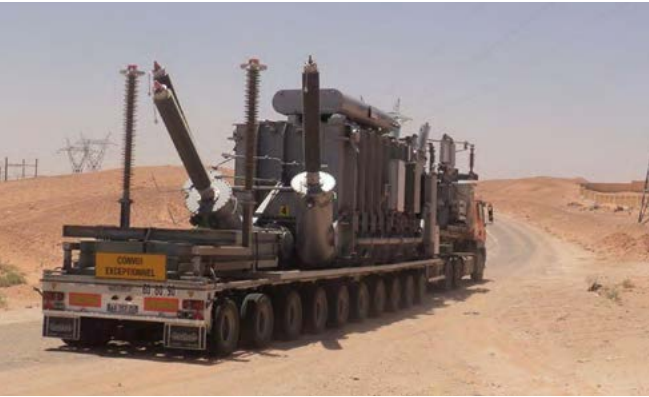
Fig. 2.4-10: 245/60-30 kV 40MVA mobile substation: Transformer trailer
