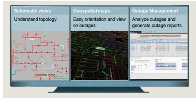
Fig. 7.1-33: Distribution SCADA, outage management and advanced fault and network analysis operated under one common user environment
