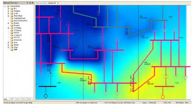
Fig. 9.4-1: Visualizing PSS®E results using single-line diagram contouring
