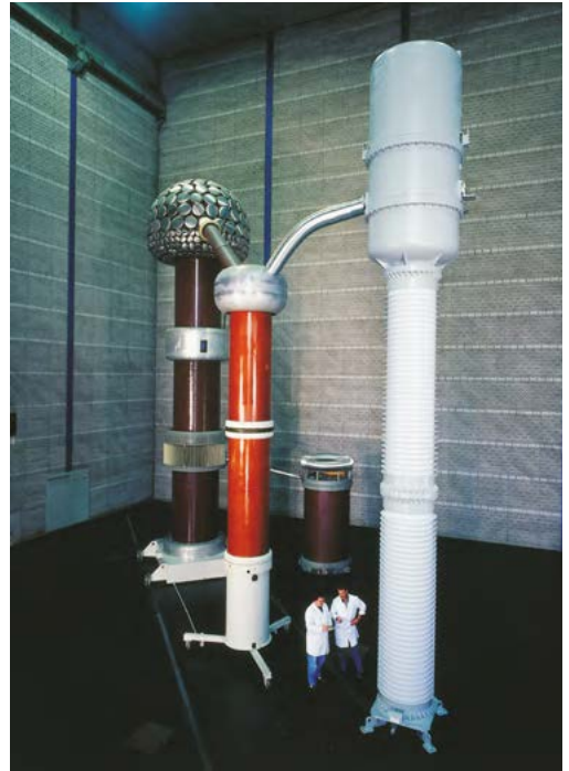
Fig. 4.2-19: 800 kV gas-insulated combined instrument transformers
