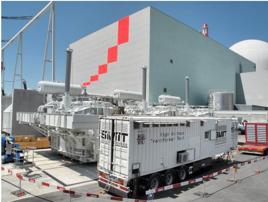
Test facility (container) with test objects and power plant
