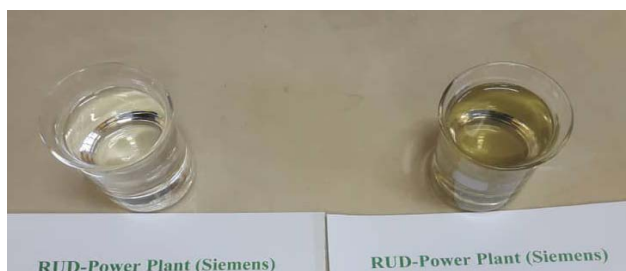
Figure 7: Right: OS3 sample with corrosive sulfur and 160 ppm DBDS Left: OS3 after treatment with modified catalyst, none corrosive and <5 ppm DBDS
